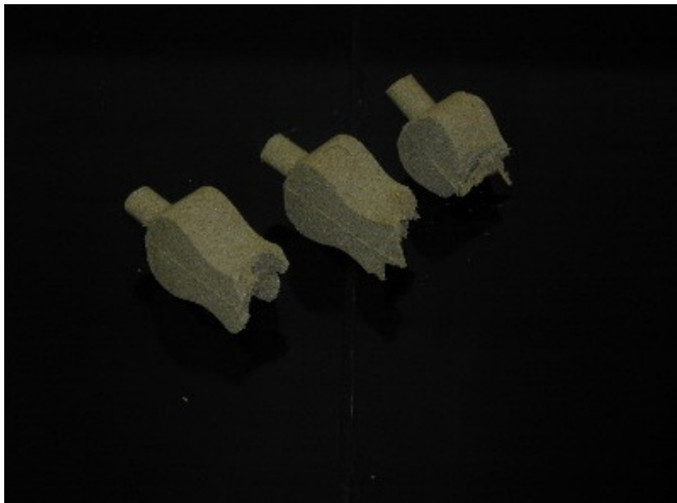
Figure 4 Weigh cure portion of the cores to measure bulk cure speed.
