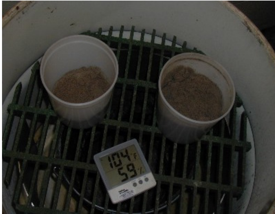
Figure 5 A bench life study with high temperature and elevated relative humidity.
