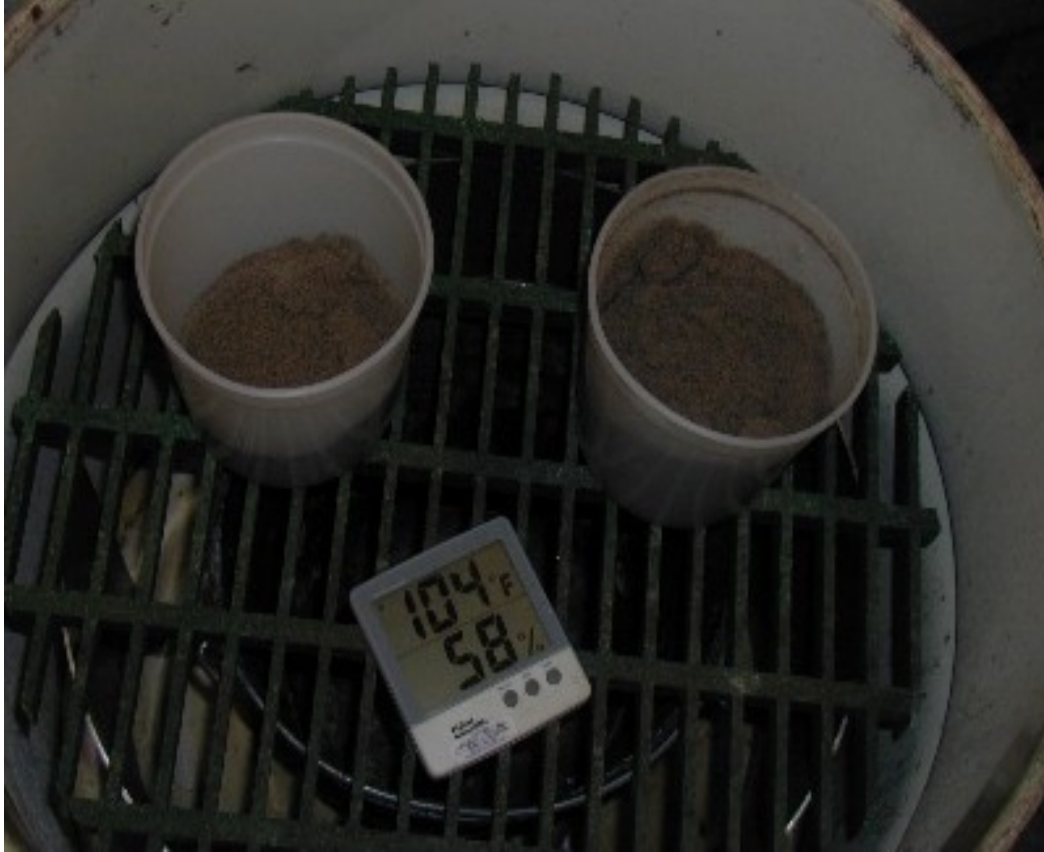
Figure 7 Humidity Chamber used to expose sand to elevated temperature and relative humidity.
