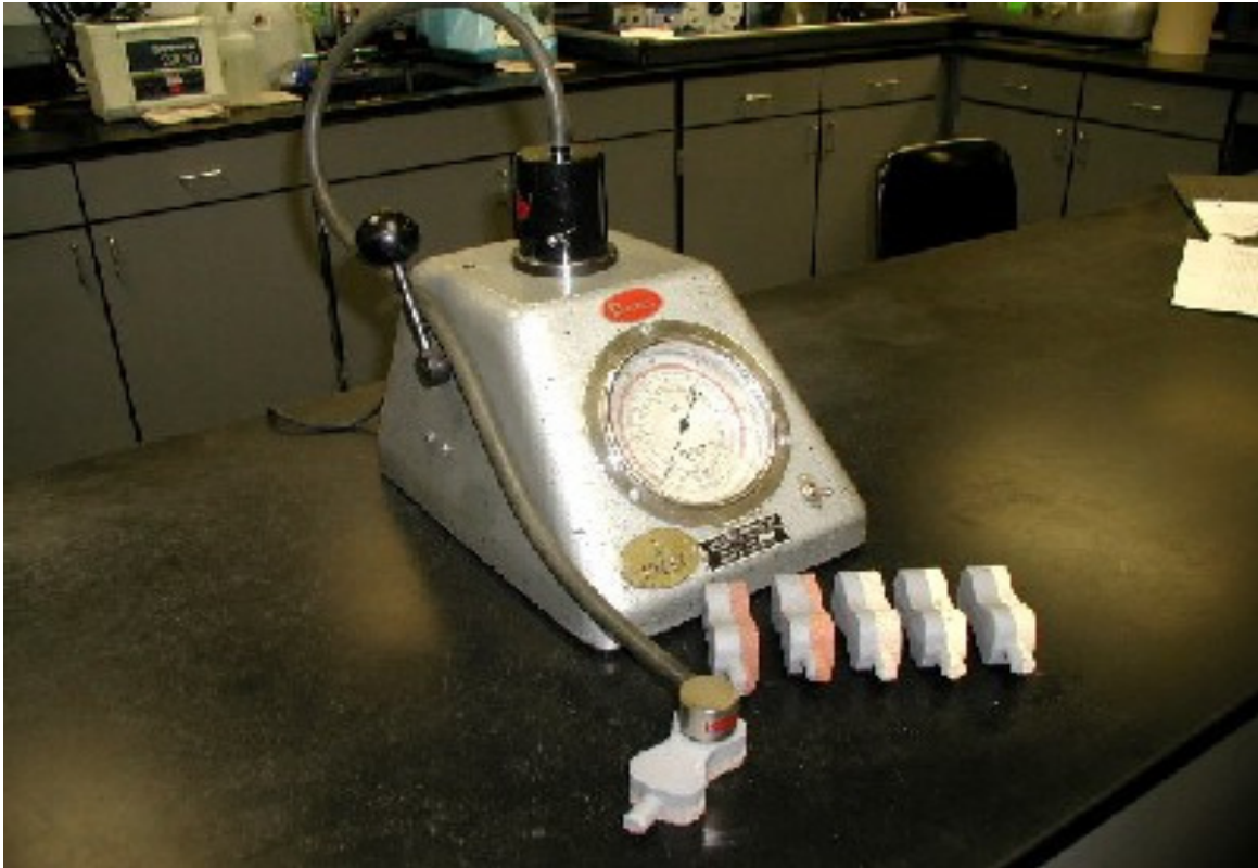
Figure 6 Measuring permeability for cores.
