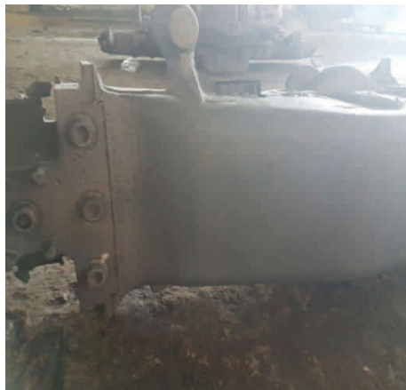
Fig.5 Casting after changing the ingate, no scab defect found.
