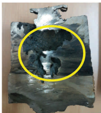
Fig.18 Shrinkage Pattern in riser after reduction of riser & Shrinkage Pattern in Simulation.
