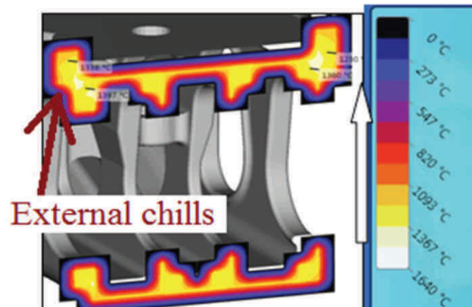
Fig.11 No hot zone (temp.1380°C).(by Auto Cast)
