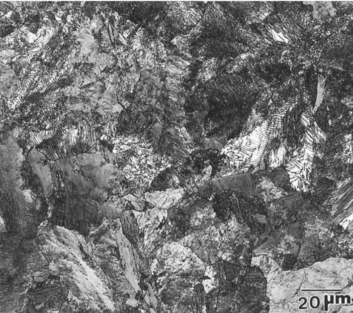
Fig. 1.4 Micrograph of ASTM A 1 rail steel showing the fully pearlitic microstructure. Etched in 4% picral. 500×
