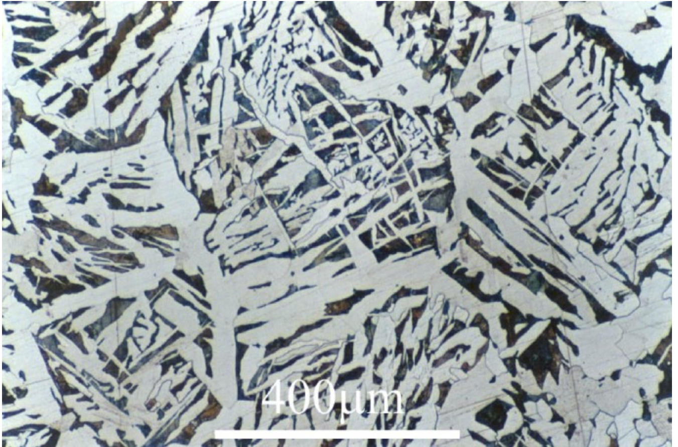
Figure 43: Mixture of allotriomorphic ferrite, Widmanstätten ferrite and pearlite. Micrograph courtesy of DoltPoms project.
