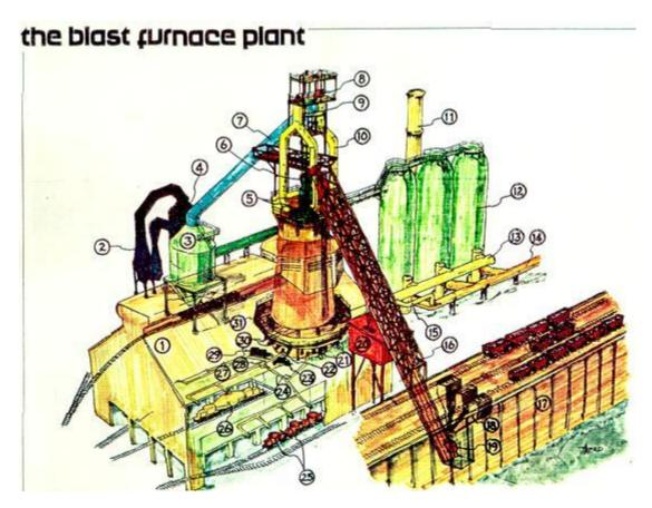
Now that we have completed a description of the ironmaking process, let s review the physical equipment comprising the blast furnace plant.
