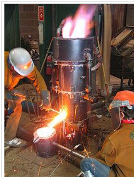
A cupola furnace in operation at Wayne State University, in Detroit, Michigan
