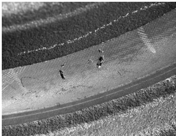
Example of Nitrogen porosity defect in grey iron revealed on machining.
