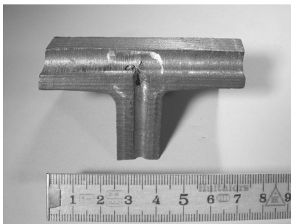
Overview of the position of the shrinkage. The defect was revealed after machining and was located in the centre of the casting section with T-shape.
