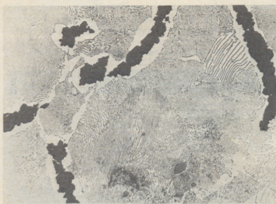
3 Compacted form of graphite associated with nitrogen fissure defects.
