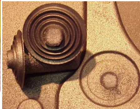
2 Collapsible Core Sleeves / Casting
