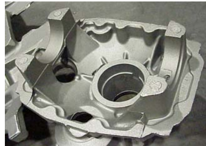
Casting after Feeder removal
