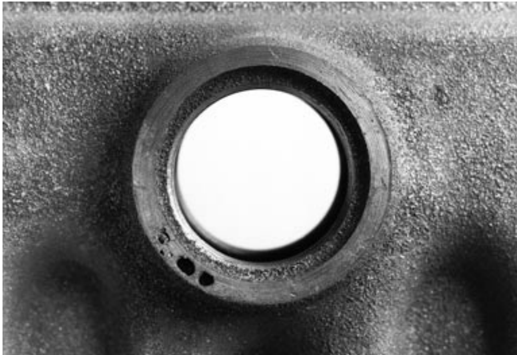
Fig. 25: Low-alloy grey iron casting. Formation of surface blowholes in the top part. Scale: 10 mm \cong 33 mm
